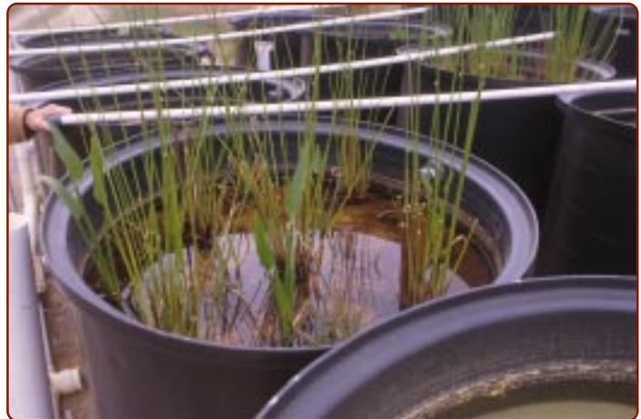
An experimental treatment wetland in D-Area on the Savannah River Site tests the ability of native aquatic plants to remediate the acidic, metal-contaminated runoff from a coal pile.
