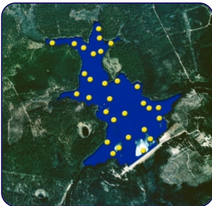
Aerial view of Pond B on the SRS, showing approximate locations of 30 sites sampled in 1984 and 1994 to determine the inventory of  $^{137}\text{Cs}$  in pond sediments.
