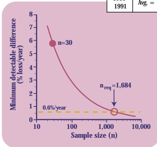
Minimum detectable difference in sediment  $^{137}\text{Cs}$  inventory as a function of sample size. The dashed line indicates the estimated export rate of  $^{137}\text{Cs}$  in surface water between 1984 and 1994. The sample size required to detect a change in the sediment  $^{137}\text{Cs}$  inventory equal to the surface water export is indicated by the open circle.
